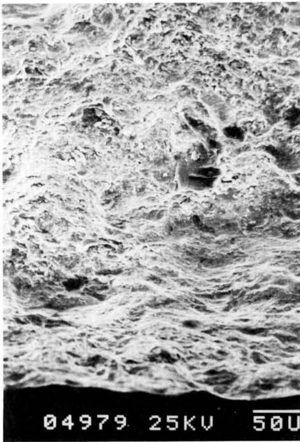
Fig. A3—The worn surface of the mild steel (left) and an 11° polished section of the 'white cast iron'
